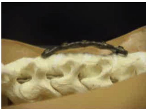
Fig. 30. An anterior cervical plate following 3-point bending resting on top of a model cervical spine for comparison of the curvature obtained from the bending.
